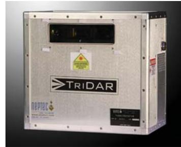
sensor head, drastically reducing the computational overhead of working in 3D. The result is six degree-of-freedom (6DOF) real-time tracking and pose estimation.
