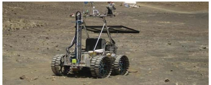
The rover can be controlled directly through an RF-handheld transmitter, tele-operated remotely through a Remote Control Station (RCS), or can be commanded to autonomously navigate and avoid obstacles using an onboard suite of vision and navigation sensors. The RF-handheld transmitter provides basic control of the rover driving functions as well as chassis pitch and brake controls.
